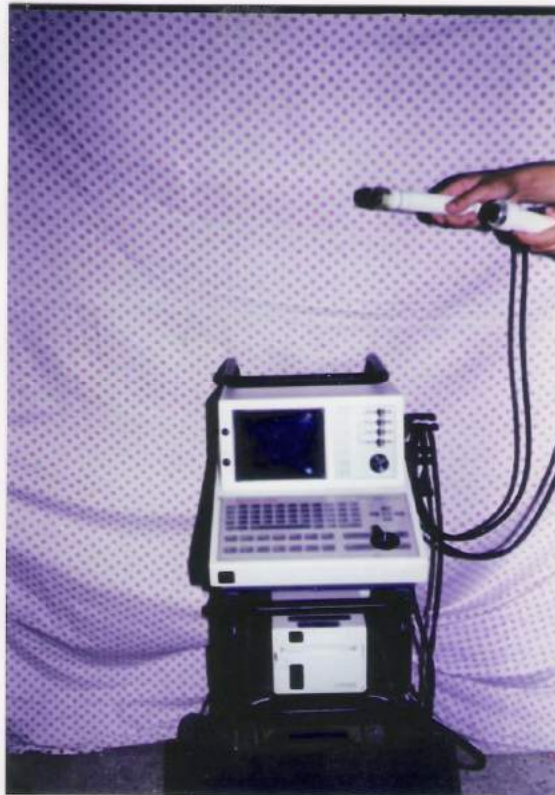
Fig. (3): PIE- Medical 150 Scanner with MITSUBISHI thermal video - printer and 5.0/7.5 MHZ transrectal and 3.5 transabdominal transducers.
