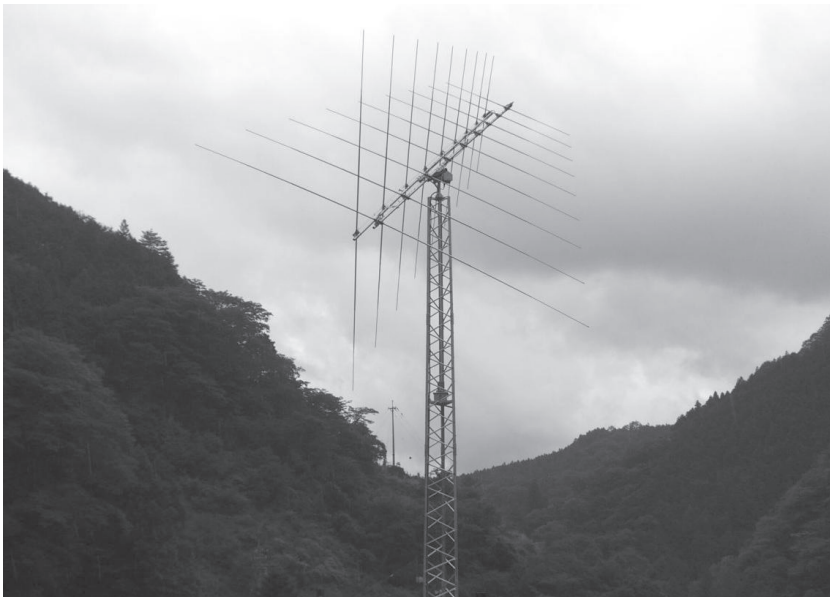
Figure 8.9. The log periodic antenna of Agawa Jovian Radio Observatory of Kochi National College of Technology.
