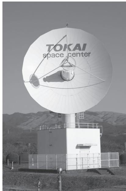
Figure 8.5. The 11 m single dish of Tokai University.
