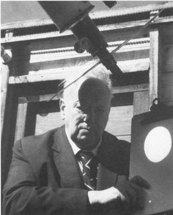
Figure 3.7. Patrick Moore shows how to use a simple hand-held screen for solar projection.
