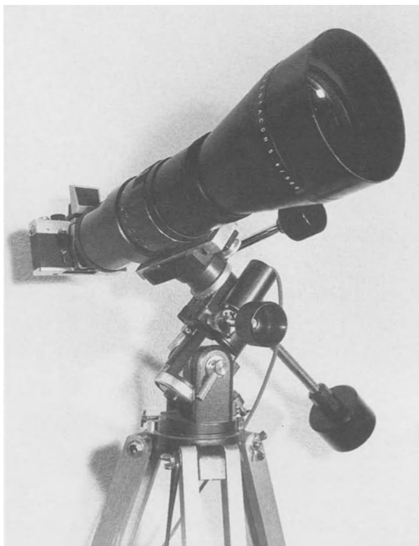
Figure 8.2. A typical tripod and head arrangement. (Michael Maunder)
