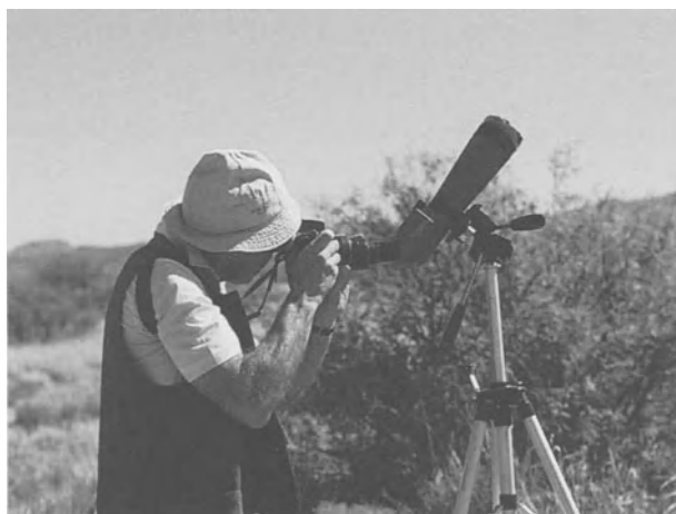
Figure 7.5. A telescope with camera attached at right angles for afocal projection. Arizona, 1994.
