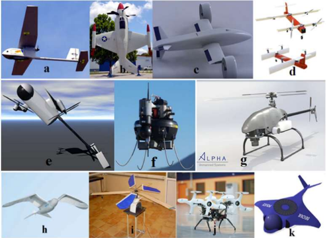
Different types of \mu UAVs, (a) HTOL (b) VTOL (c) tilt-rotor (d) tilt-wing (e) tilt-body, (f) ducted fan \mu UAV (g) helicopter (h) ornithopter (i) ornithopter (j) cyclocopter and (k) unconventional \mu UAV
