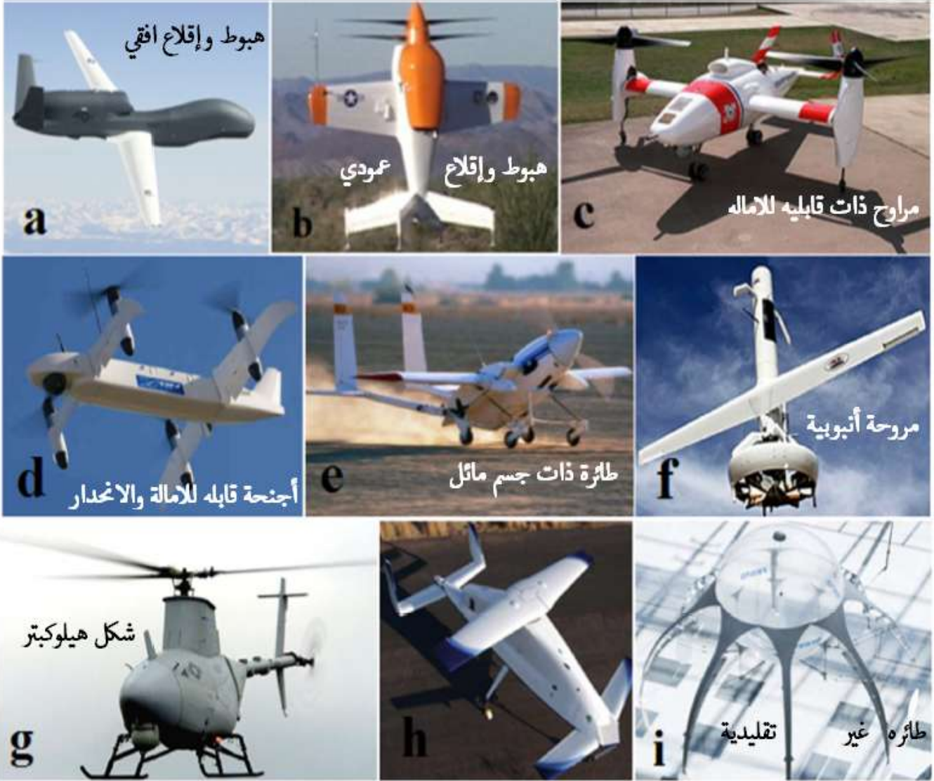
Different types of UAVs, (a) HTOL (b) VTOL (c) tilt-rotor UAV (d) tilt-wing UAV (e) tilt-body UAV (f) ducted fan UAV (g) helicopter (h) heli-wing and (i) unconventional UAV
