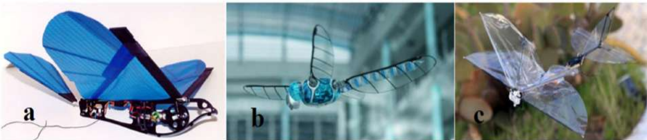
Fig. 6. Different configurations of FWMAVs, (a) monoplane, (b) tandem, and (c) biplane [112].
