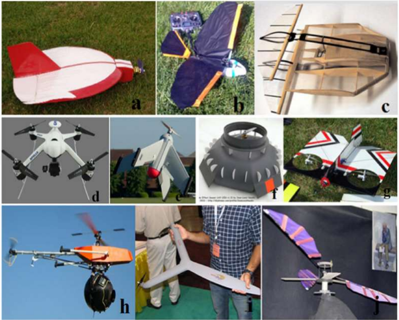
Fig. 5. Different types of MAVs, (a) fixed wing [6], (b) flapping wing [83], (c) fixed/flapping-wing [84], (d) rotary wing [85], (e) VTOL [86], (f) ducted fan [87], (g) tilt-rotor, (h) helicopter [88], (i) unconventional, (j) ornicopter [89].
