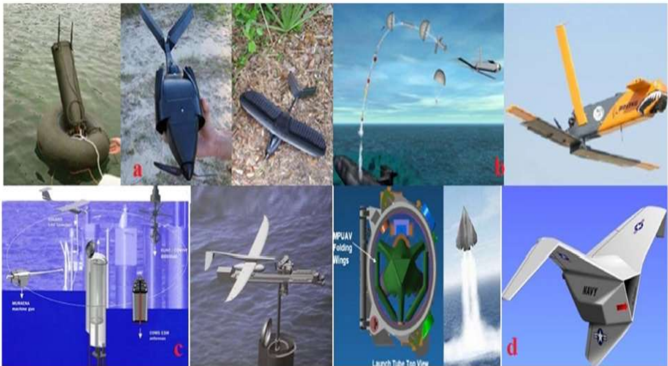
Drones' in marine environments, (a) TacMAV [209], (b) Scan Eagle [210,211], (c) Volans [212,213], and (d) Cormorant [214,215].
