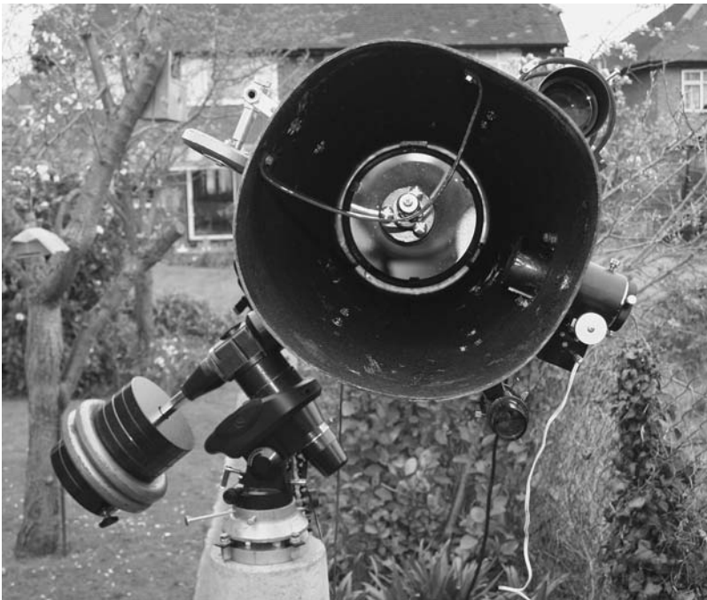
Figure 10.4. Looking exactly down the optical axis of a precisely collimated f4.8 Newtonian (secondary in line with its reflection), the offset of the secondary away from the focuser is clear.
