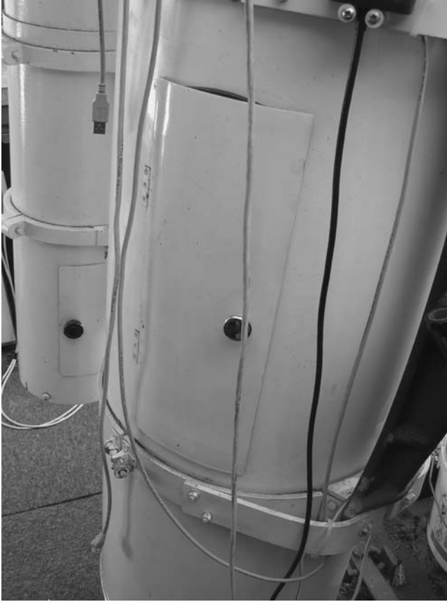
Figure 9.6. Home-built cradles and door in the tube of the 350 mm (14 in.) reflector.
