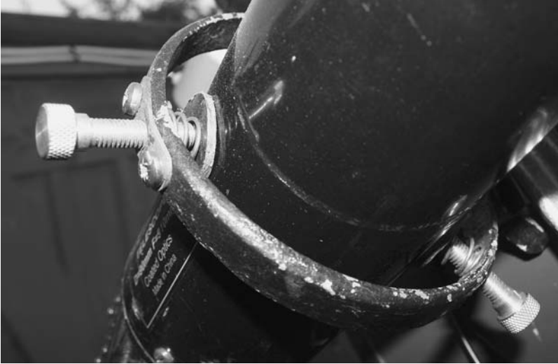
Figure 10.12. Guidescope ring modification with springs and plastic disks.
