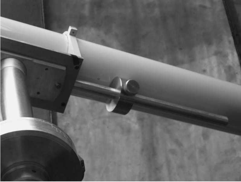
Figure 9.39. Adjustable counterweight and bar on the saddle plate.
