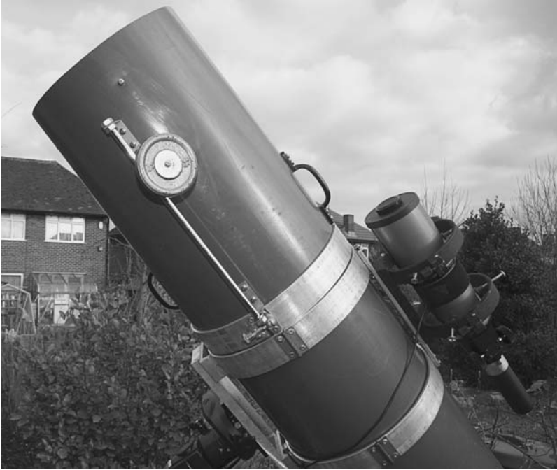
Figure 8.1. My Newtonian with a rotatable tube and handles. The small telescope stays fixed. Note also the sliding weight.
