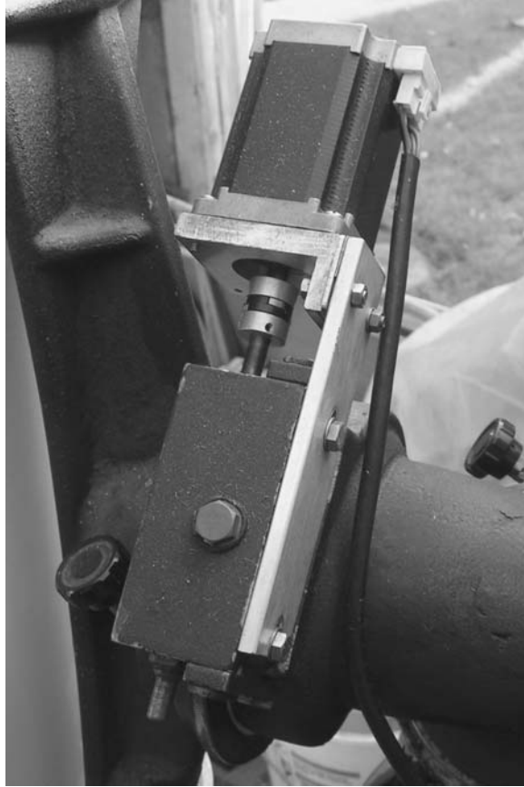
Figure 9.7. New stepper motor and bracket on the Fullerscopes mount.
