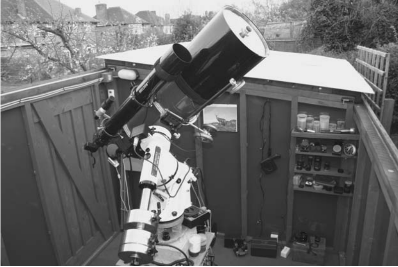
Figure 9.27. General view of the run-off roof shed, with the Cassegrain on its new mounting.
