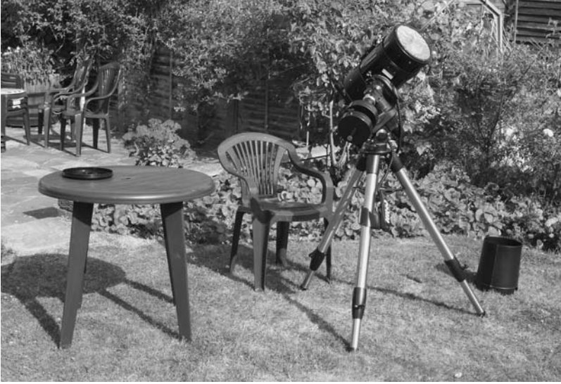
Figure 3.1. Basic minimum observatory, with a 20 cm (8 in.) SCT set up on a lawn, with plastic table and chair, and rigid dew-shield, not fitted.
