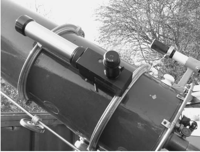
Figure 1.5. Small solar telescope mounted with a much larger telescope. It is attached with just a camera tripod screw.
