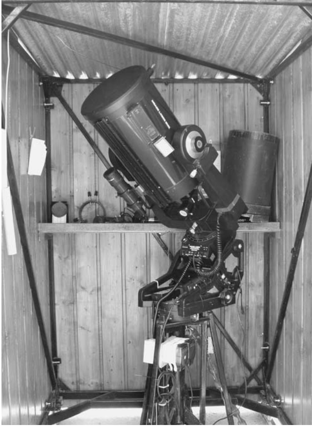
Figure 9.13. The inside of the SCT run-off shed.
