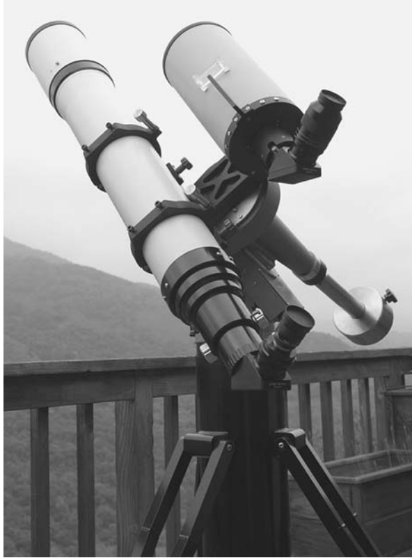
Figure 10.15. Side-by-side balanced arrangement of two telescopes mounted on a tandem bar (Astro Accessories from RobinCasady.com).
