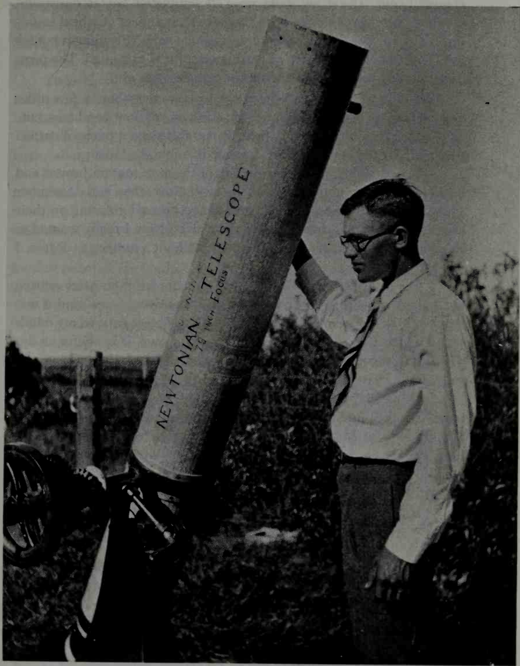
Clyde W. Tombaugh, at the age of twenty-two, with his homemade 9-inch (22.9-centimeter) reflecting telescope on the family farm near Burdett, Kansas. This picture was taken in the summer of 1928, eighteen months before the discovery of Pluto.
