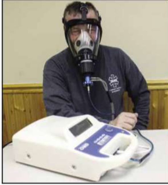
A firefighter undergoing SCBA facepiece fit-testing.
