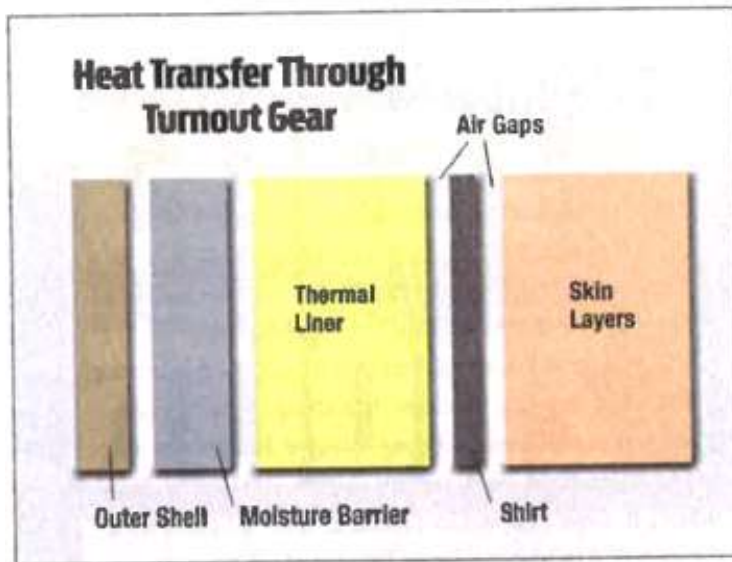
Multiple barriers and air gaps exist between the fire and the firefighter's skin.
