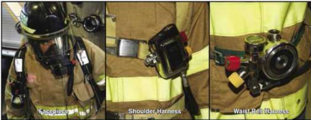
On modern SCBAs, the regulator attaches to the facepiece while on older models it was located on the shoulder harness or waist belt harness.
