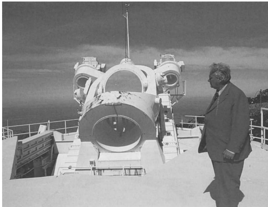
Figure 16.2. The heliostat of the McMath solar telescope is capable of projecting a solar image down into this tunnel where observing conditions underground are much more stable.
