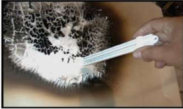
(b) Measuring Depth of Calcination on a Piece of Gypsum Wallboard.
