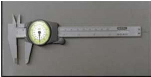
(a) Dial Calipers with Depth Probes.
