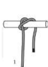
Round Turn and Two Half Hitches
